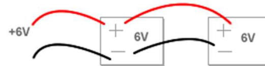
Connecting in Parallel (same voltage, double capacity [ah])
